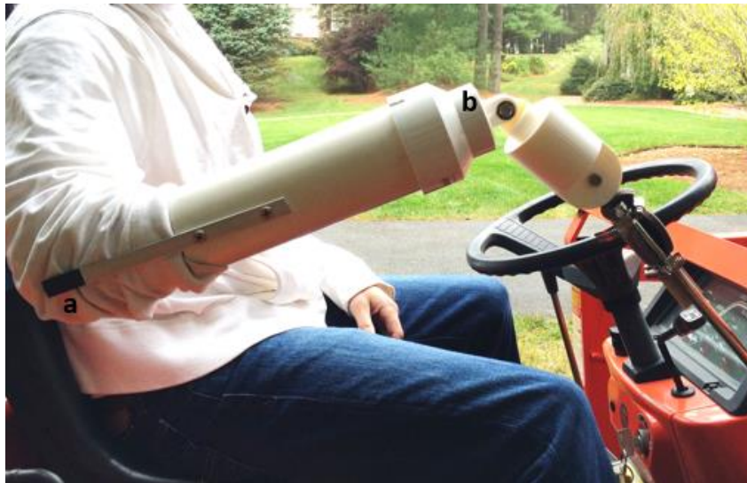
Figure 23: First iteration of test fixture in use on Kubota tractor
