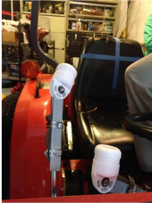
Figure 28: Setup of adapters on hydraulic lever and throttle
