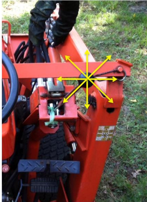
Figure 12: Tractor hydraulic lever and its approximate range of motion
