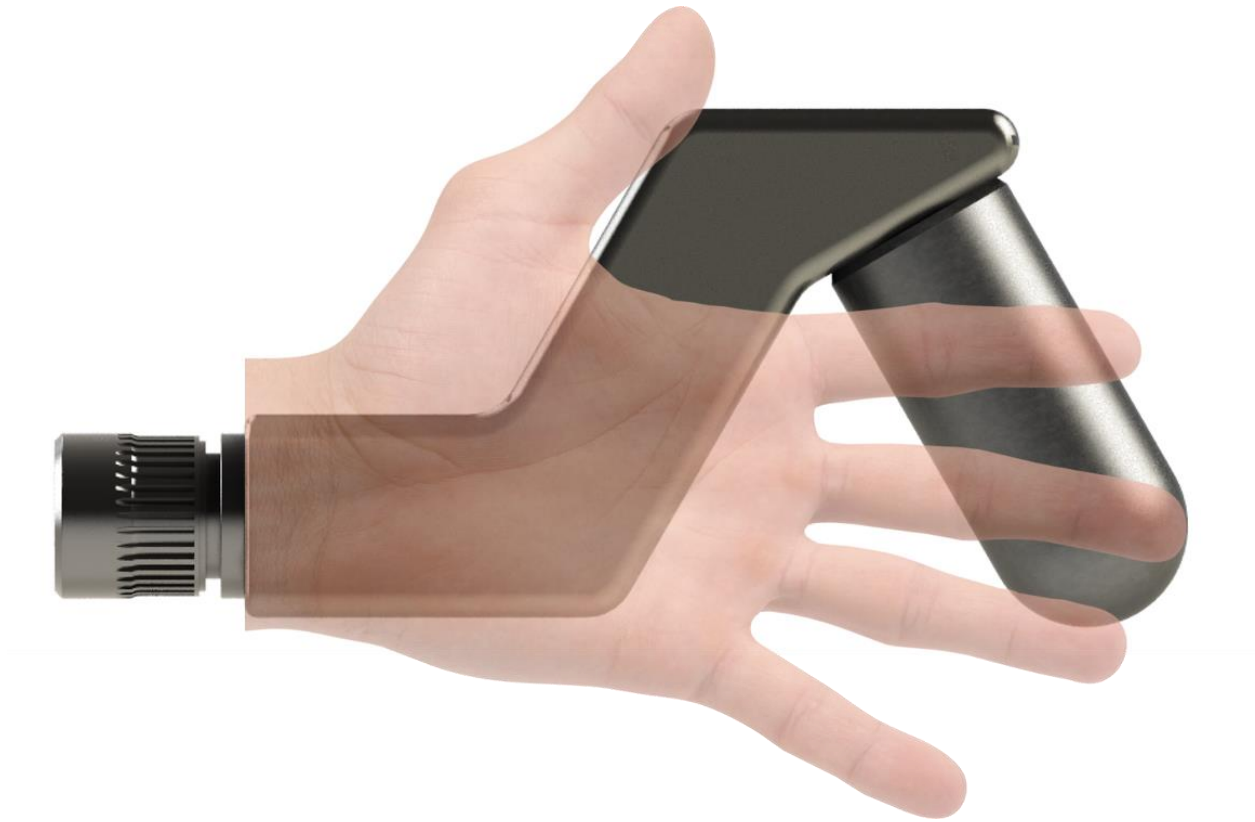
Figure 17: Terminal device with translucent overlaid average hand size showing positioning of mating surfaces with respect to the wrist
