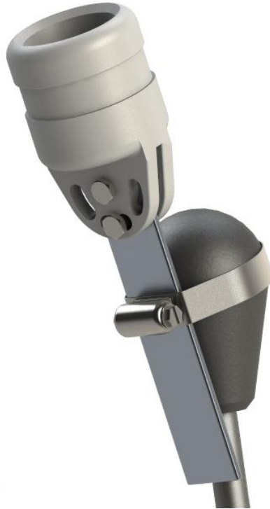
Figure 19: Model of adapter connected to tractor control using off-the-shelf hardware
